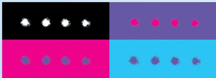
Trapped barium-133 ions, imaged with laser-induced fluorescence.
