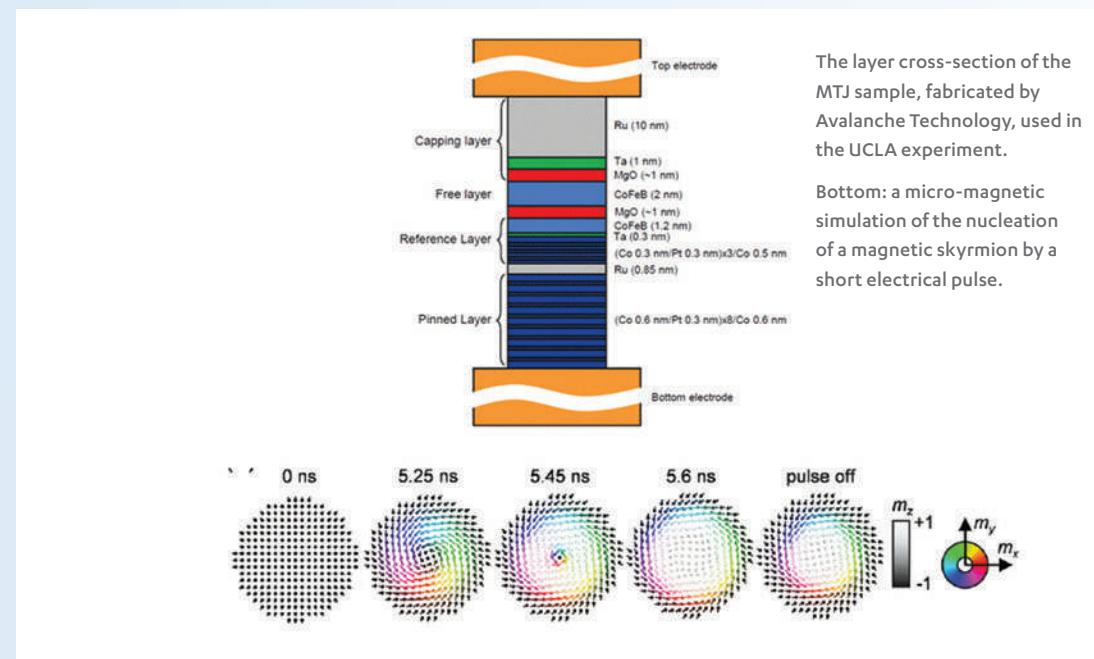
The layer cross-section of the MTJ sample, fabricated by Avalanche Technology, used in the UCLA experiment.
