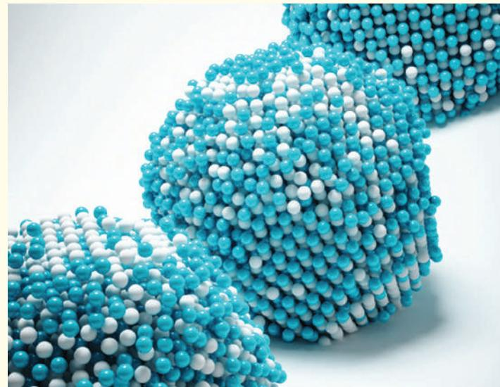
This image shows atomic electron tomography captures 4D atomic motion in an iron-platinum nanoparticle at three different annealing times.
