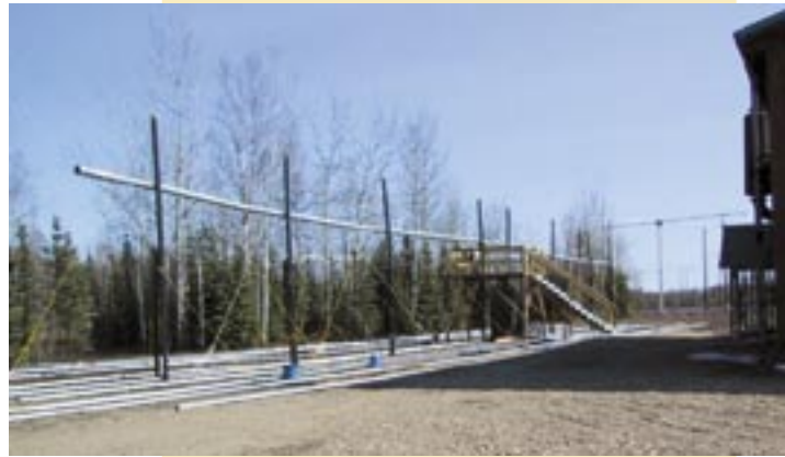
Photograph of the 2.85 MHz Hertzian antenna at HIPAS, April 2003. This antenna is 104 meters long and 5 m above a ground plane made up of 2-1/2 inch diameter aluminum pipes. The antenna is supported by 4-inch diameter PVC drainpipe. It has a capacitance of 200 pF across its spark gap. The stairways are for central access. One of the antennas of the CW array at HIPAS is seen in the background
