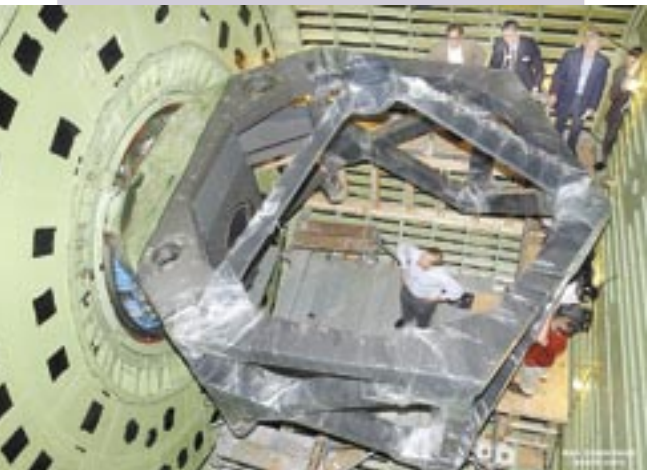
A wide-angle view of the SOFIA telescope through the aircraft opening. The telescope carbon fiber metering structure, including the secondary mirror support, is now mounted on the bulkhead of the aircraft. The primary mirror was placed on the metering structure shortly after this picture was taken. U.S. House Representative Chet Edwards from Waco Texas is standing in the center of the open air cavity.
