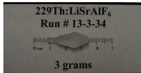
Picture of bulk ^{229}\text{Th} :LiSAF crystal, which is the result of 5 years of crystal growth work.
