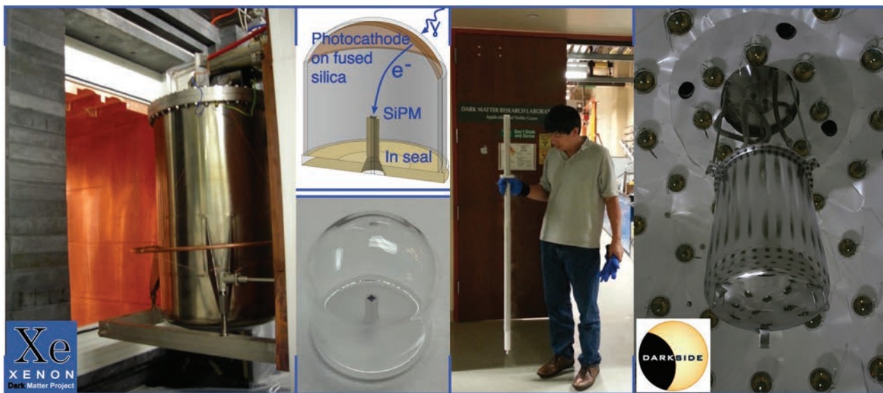
Figure 1. XENON100 detector in its shielding; (middle left): SiGHT conceptual drawing and detector structure; (middle right): Dr. Hanguo Wang in front of the UCLA lab with one of the HVFT prototypes. (right) DarkSide-50 detector inside the neutron veto.
