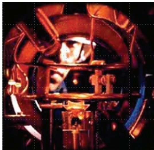
Kris Helmerson of NIST looking into a vacuum chamber at a sodium MOT. The sodium atoms, visible as the bright orange dot in the middle of the picture, are cooled and levitated by lasers.
