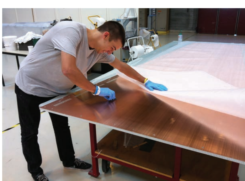
UCLA undergraduate Jacob Beres works at CERN preparing copper-clad panels for building new muon detectors. UCLA is helping build the upgrade of the Compact Muon Solenoid Experiment for the higher energy and higher luminosity running of the Large Hadron Collider scheduled to begin in 2015.
