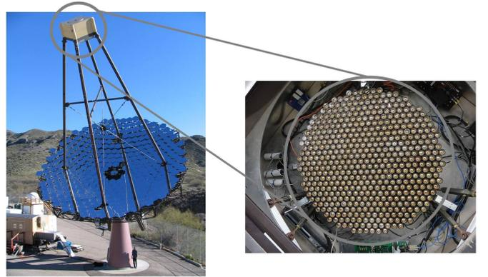
FIG. 3: Each of the four VERITAS telescopes consists of a 12m reflector comprised of 350 mirror facets, which focus light onto a camera with 499 pixels.
