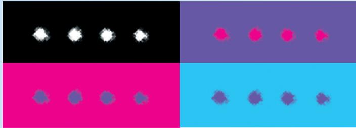
Trapped barium-133 ions, imaged with laser-induced fluorescence.
